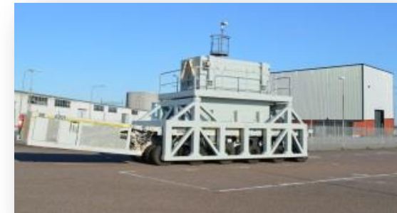
Photo: BKAB. On site transportation of RPV internals to interim storage.
